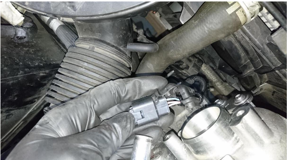
The intake pipe is also designed in a way that you can't accidentally fit the wrong turbo. With a hack saw or a cutting disc you just need to remove a small piece of plastic to allow the pipe to clamp down flat to the turbo inlet.
