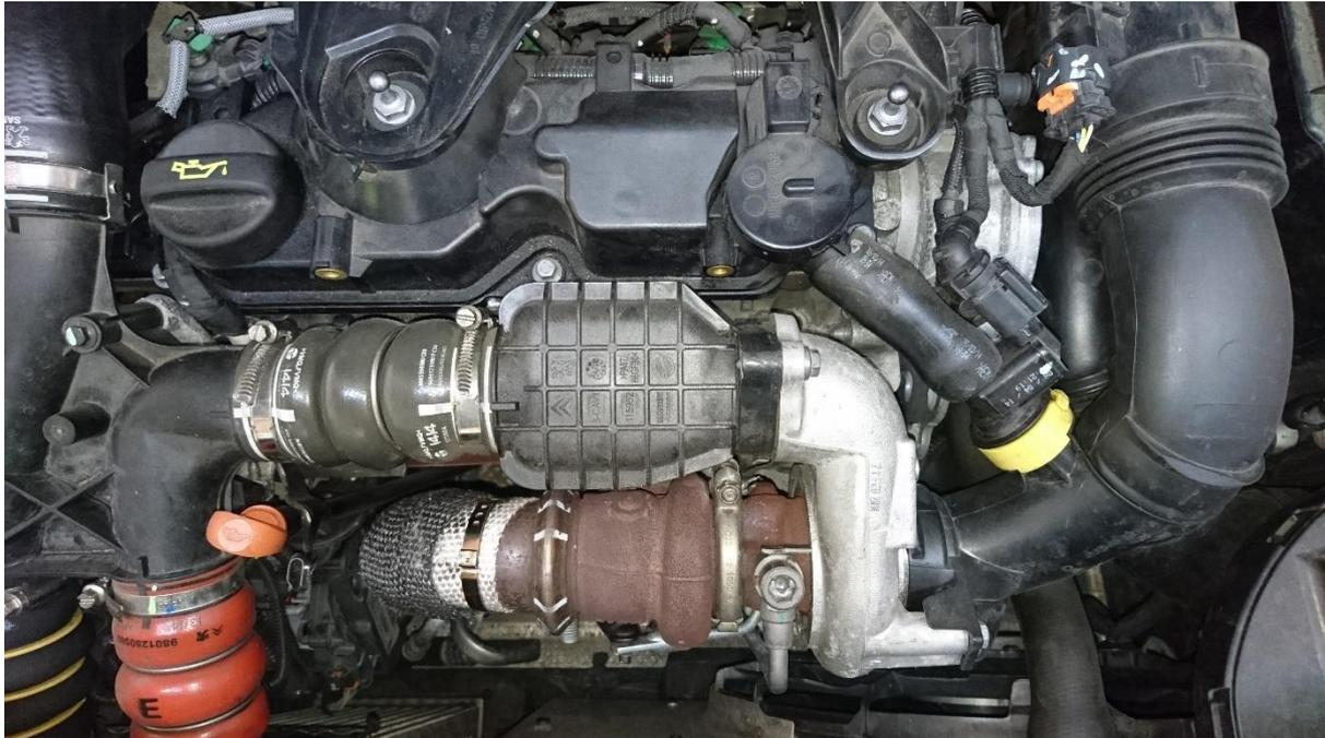
Remove the intake pipe which is held on with a 10mm bolt, and the turbo outlet to intercooler pipe which has two 10mm bolts and the jubilee clip uses a 7mm socket.
