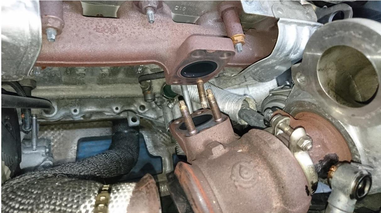
Before you refit the turbo, you will need the correct oil pipe (part number 63846), as shown here the pipe for the GTD1244VZ is completely different. I would also recommend fitting new banjo bolts. Don't remove the strainer from the lower bolt, it's a filter and an oil restrictor, removing it will cause future problems.
