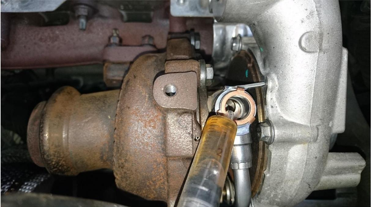
When you come to connect the plug to the turbo actuator position sensor you will find that it has been designed to prevent you from connecting it to the wrong turbo. To get the extra length on the wire you simply need to remove the 90-degree collar that is clipped on to the wire.
