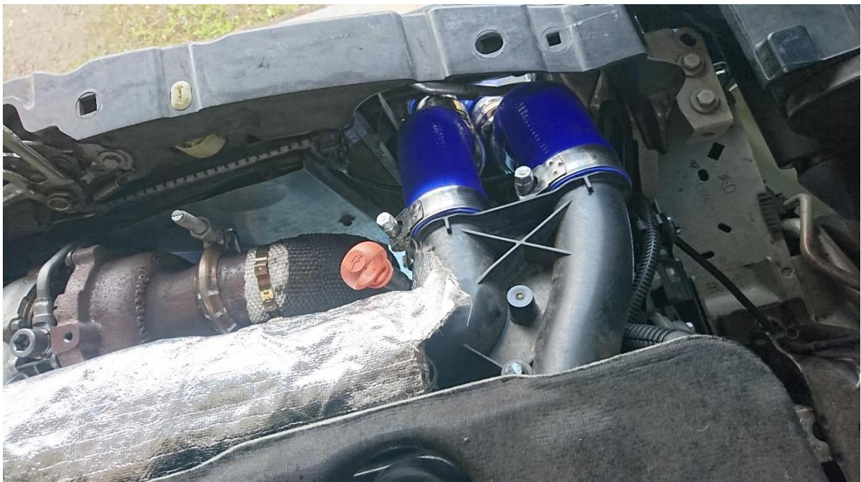
Here's the final job with the intercooler and pipe work fitted.
