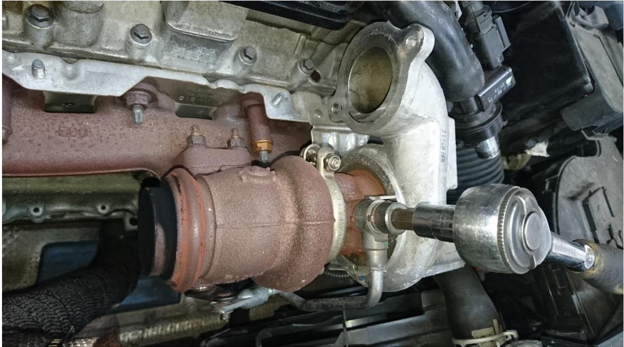
The next step is to loosen the 4 11mm nuts holding the turbo to the manifold. If these are tight you might want to join two spanners together to get some extra leverage.
