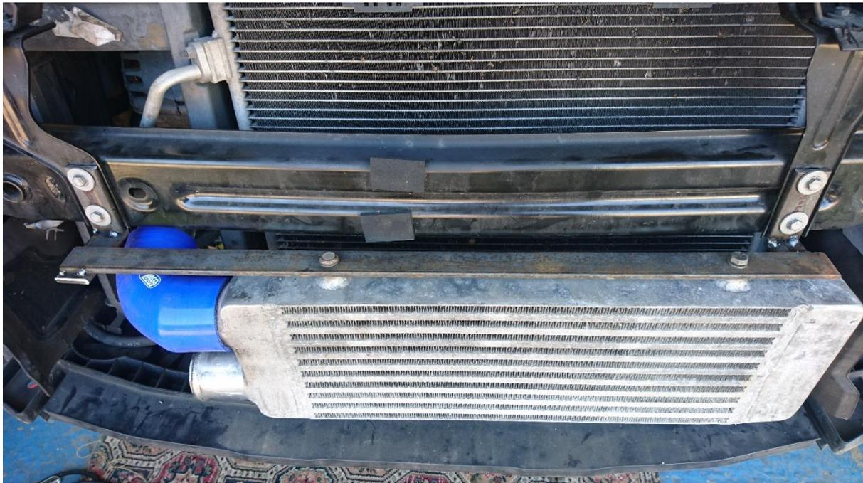
Once you're happy the bracket is the correct size and that the bumper will fit back on you can weld it fully and paint it to prevent rust.
