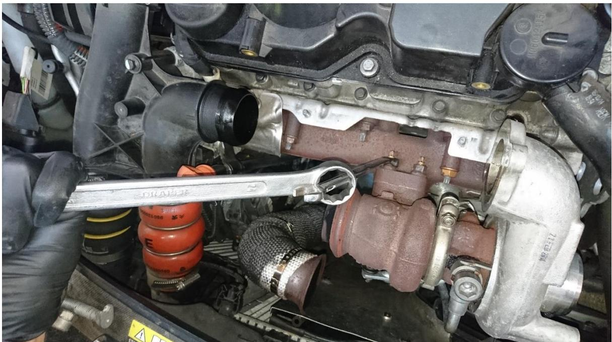
With the four nuts off you can slide the turbo outwards and then you'll be able to easily see the turbo oil drain. Loosen the 7mm nut on the jubilee clamp and then pop the hose off. The turbo will now come out.
