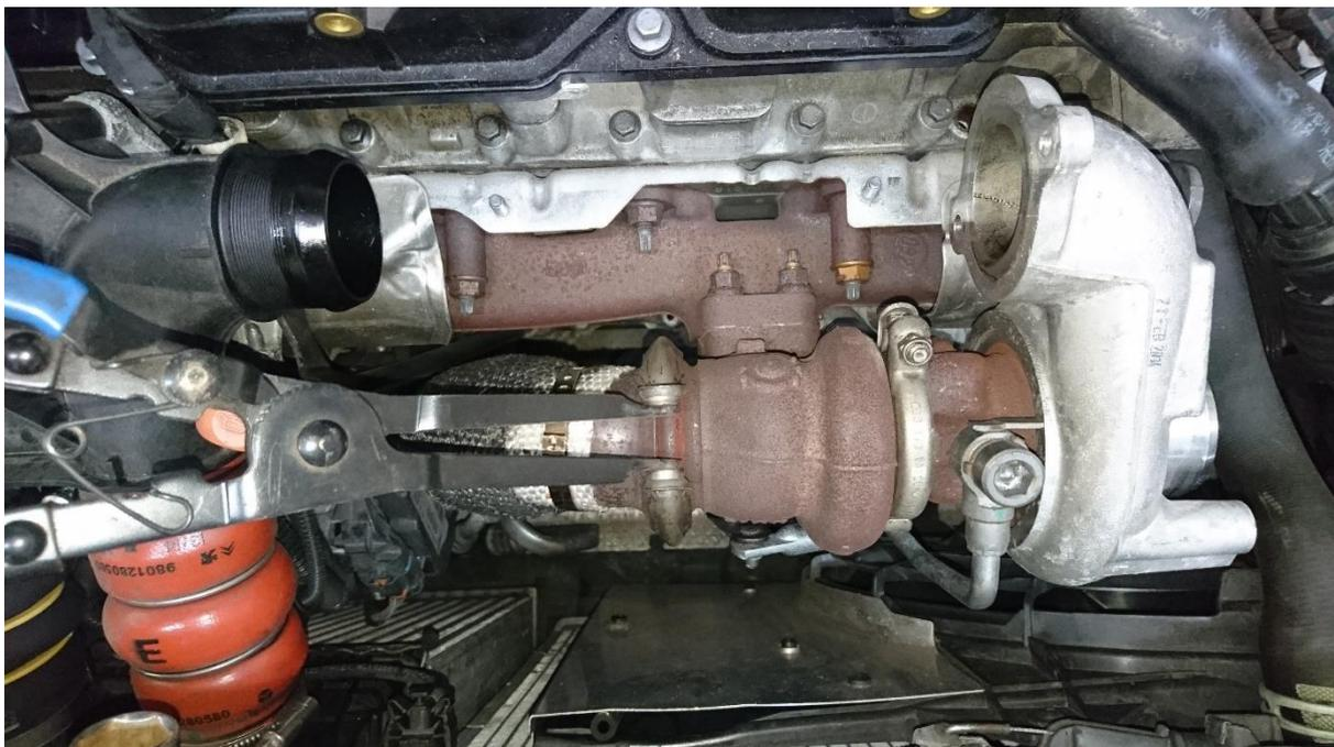
The exhaust clamp uses a 16mm nut at the bottom and then you can use a tool as shown above to remove the v band clamp.
