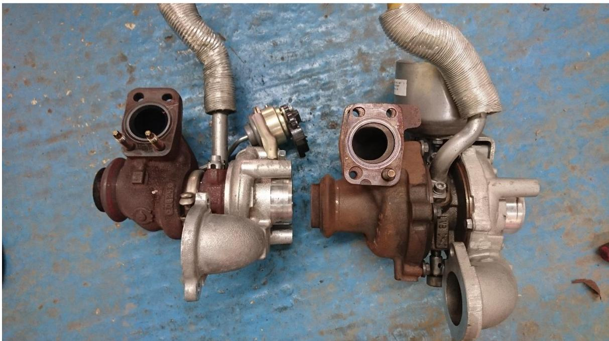
The position of the oil drain and the oil feed is the same, so it's quite an easy conversion.
